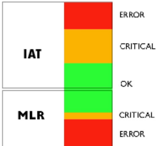
Typical MediaWindow scale of an IAT/MLR measurement
